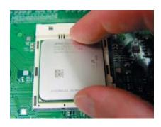
4. With the CPU inserted into the socket, inspect the four corners of the CPU to make sure that it is properly installed and flush with the socket.
